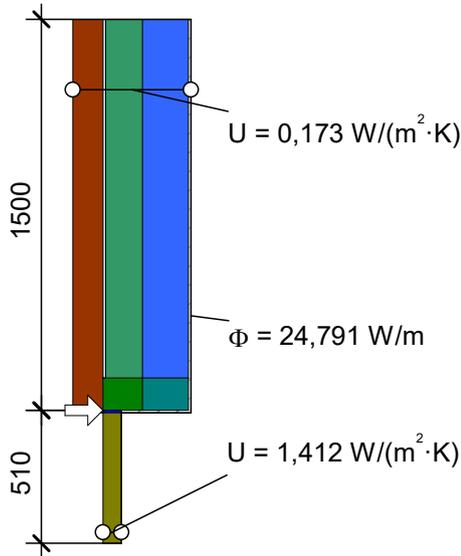
Abmessungen in mm
